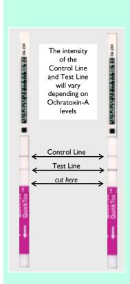
Cut strip and place in QuickScan reader immediately no drying step!
